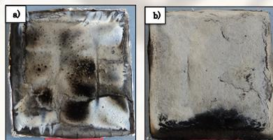
Fig. 5 - Cone calorimeter residues of (a) A-LOIopt and (b) B-CCTopt.
